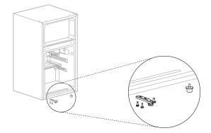
**06** Place refrigerator door on bottom hinge, then fix the middle hinge on the left side and insert the hole caps on the right side.
