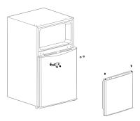
**07** Place freezer door on middle hinge, then fix the top hinge, top hinge cover on the left side and insert hole caps on the right side.
