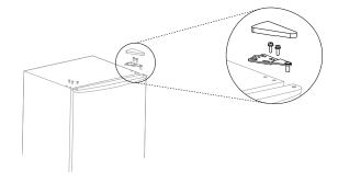
**03** Remove freezer door as well as middle hinge and hole cap of the other side;
