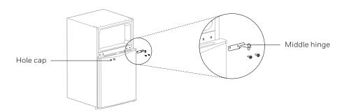
**05** Exchange the installation position of bottom hinge and adjustable foot, then fix them respectively. Remove the hinge sleeve pipe of the refrigerating door, and install it on the other side. Remove the hinge sleeve pipe of the freezer door and install it on the other side.
